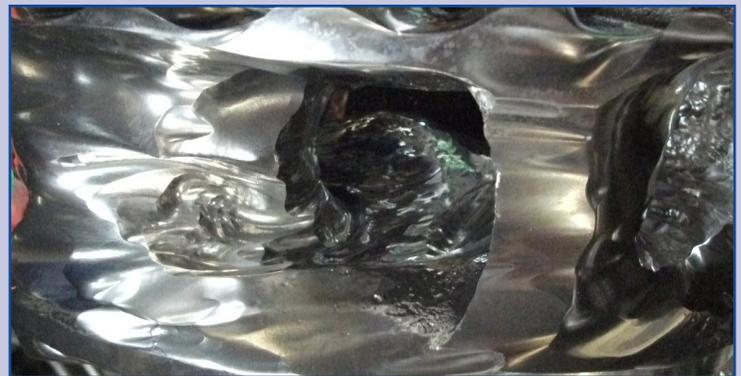
*Impeller scoured by the sand mixture*
